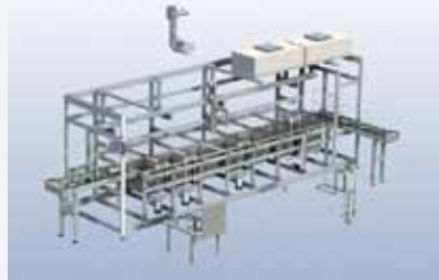
Ultrasonic cleaning lines composed of modular components
